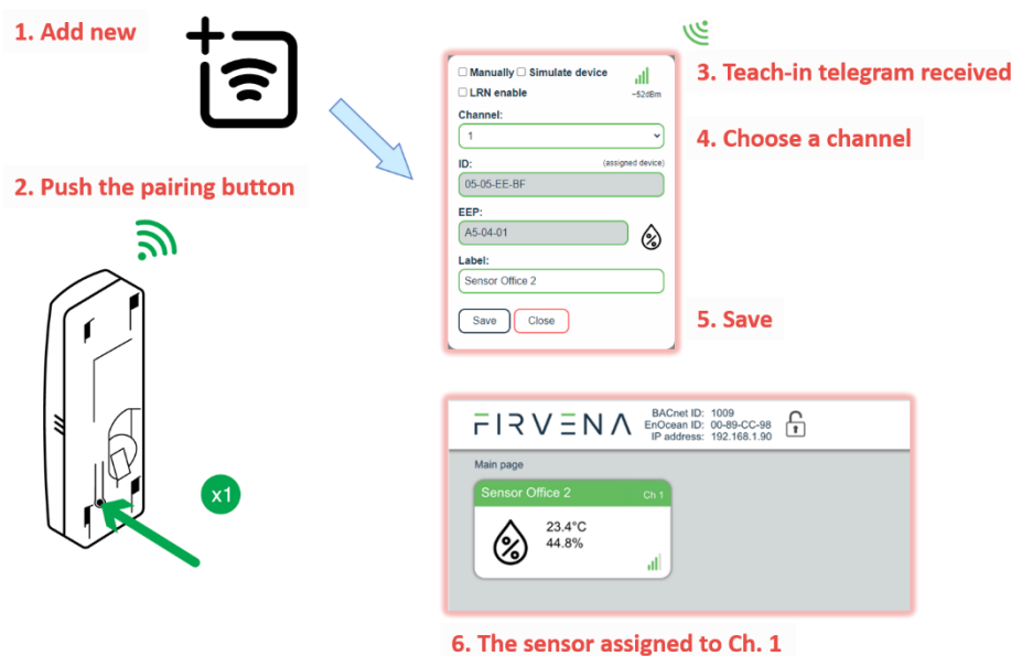
Fig. 5.2 Adding elements – teach-in procedure
