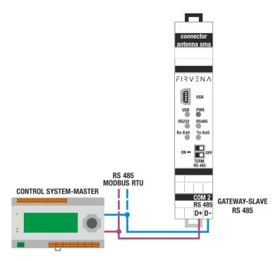
Note: If communication does not run on RS 232, RS 485, we recommend swapping the wires for RS 232 (Rx with Tx) or for RS 485 (D+ with D-) due to different specifications by control system manufacturers.
