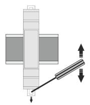
The gateway is most commonly installed into the control cabinet on a DIN rail. The gateway is fixed to the DIN rail by using plastic locks which are located on the top and bottom. See the picture. The gateway is delivered including external antenna with 2 m long cable and magnetic base which is installed outside the control cabinet.
