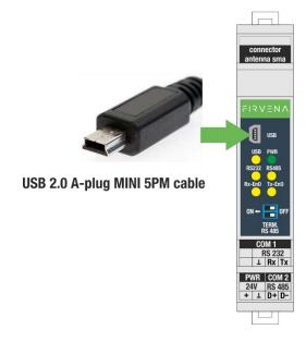
Note: For testing purposes and settings, the gateway can be powered via USB.
