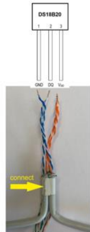
Pic. 3: Shielded cable with twisted pairs
