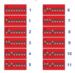
Example of setting the RS 485 baud rate:
